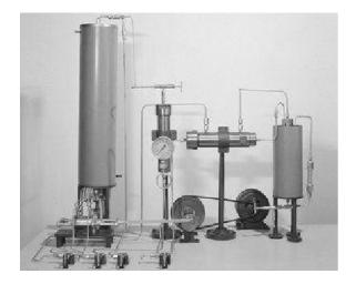
Haber reacted small amounts of nitrogen and hydrogen in a closed system to make ammonia. The reaction is exothermic.
